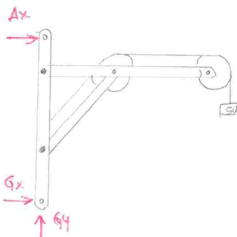
$$\begin{aligned}\sum F_x &= 0 \Rightarrow Ax + Gx = 0 \\ \sum F_y &= 0 \Rightarrow Gy - 50 = 0 \\ Gy &= 50 \text{ N} \\ \sum M_G &= 0 \Rightarrow -Ax[2,2] - 50[2,2] = 0 \\ Ax &= -50,00 \text{ N} \\ Gx &= 50,00 \text{ N}\end{aligned}$$
