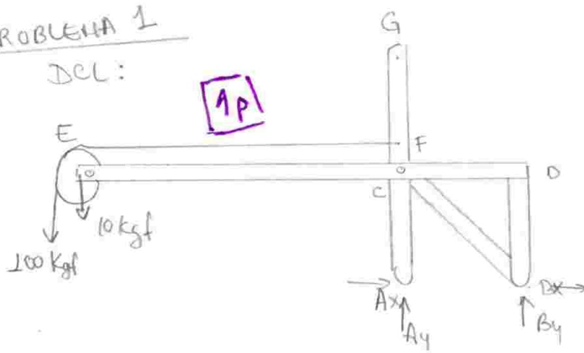
$$\begin{aligned} \text{① } \sum F_x &= 0 \Rightarrow A_x + B_x = 0 \\ \text{② } \sum F_y &= 0 \Rightarrow A_y + B_y - 100 - 10 = 0 \\ \text{③ } \sum M_A &= 0 \Rightarrow B_y(2) + 10(4) + 100(4.5) = 0 \\ B_y &= -245 \text{ kgf} \quad 1P \\ \text{④ } A_y &= 355 \text{ kgf} \quad 1P \end{aligned}$$
