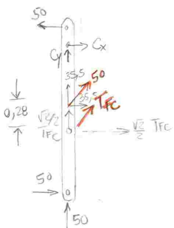
$$\begin{aligned}\sum F_x &= 0 \Rightarrow 35,5 + \frac{\sqrt{2}}{2} T_{FC} + Cx = 0 \\ 35,5 + \frac{\sqrt{2}}{2} T_{FC} + 50 + Cy &= 0 \\ \sum M_C &= 0 \Rightarrow 50[4,6] + \frac{\sqrt{2}}{2} T_{FC}[1] + 35,5[0,72] + \\ &+ 50[0,6] = 0 \\ T_{FC} &= -191,71\end{aligned}$$
